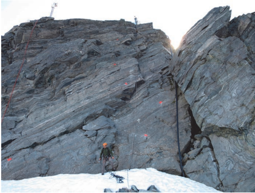
Figure 1. 20 m high back scarp of the Mannen rock slope instability with marked points of sample location for cosmogenic nuclide dating.
